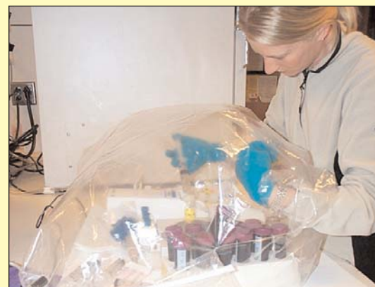
USGS's Jennifer Agee sampling sediment in an anoxic glove bag. Photo: Mark Marvin-DiPasquale
